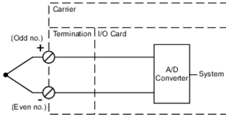
Simplified circuit and connection diagram for simplex AI card, 8-channel, 4 to 20 mA, HART.
