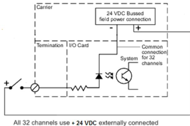
Simplified circuit and connection diagram for simplex DI Plus Card, 32-channel, 24V DC, Dry contact.
