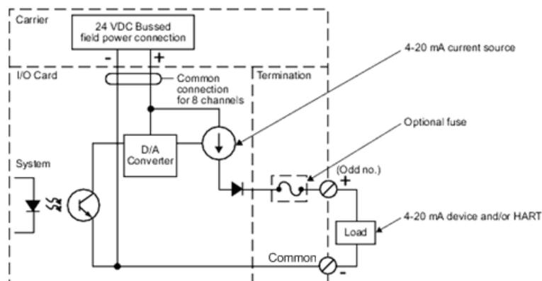
Simplified circuit and connection diagram for simplex AO card, 8-channel, 4 to 20 mA, HART.
