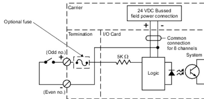
Simplified circuit and connection diagram for DI card, 8-channel, 24V DC, NAMUR/Dry Contact.
