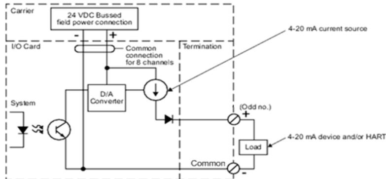
Simplified circuit and connection diagram for simplex AO (Plus) card, 16-channel, 4 to 20 mA, HART.
