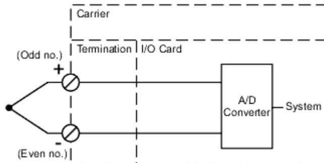
Simplified circuit diagram of Thermocouple/mV card, 8 channels.
