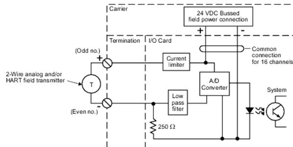
Simplified circuit and connection diagram for simplex AI card, 16-channel, 4 to 20 mA, HART.
